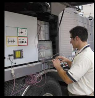
While a Putzmeister service technician does not have to be on site to view and interact with your machine's Ergonic system, relevant data can be accessed by connecting the machine directly to a laptop computer. This enables software updates and new Ergonic modules to be installed very quickly.
