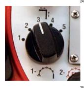
3 Semi-automatic folding in/out of the boom
