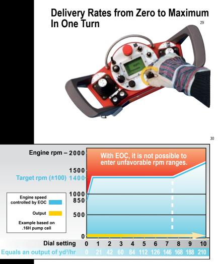
Electronics in the EOC system regulate the speed up to 75 percent of the maximum delivery rate to optimum fuel consumption. If a delivery rate above this level is selected, EOC increases the speed. However, the engine will not operate in a zone that cannot be controlled by EOC. It is not possible to set the full throttle engine speed and minimum delivery rate with EOC at the same time. If the boom is not moved and the pump is off, the speed drops back down to 850 rpm after 10 seconds.
