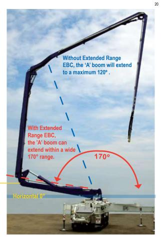
Extended Range EBC also works with our One-Sided Support (OSS) outrigger system. OSS allows the operator to reduce the machine's outrigger extension on one side, while operating within a defined working envelope.
