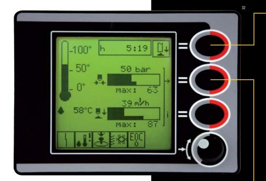
Simple to use, the EGD gives the pump operator a quick and clear visual display of important machine information as well as the ability to set individual pumping parameters.
