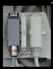
A quick plug-in connection activates Extended Range EBC for large roll-and-fold models. Simply moving the plug into the right receptacle returns the boom to routine operation.
